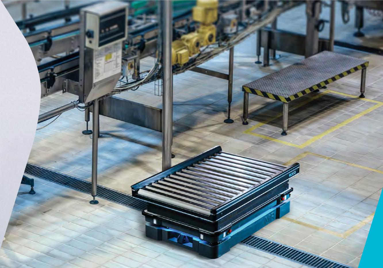
*The ROEQ TR500 Auto is ideal for transporting and transferring between conveyor lines of different heights.*
